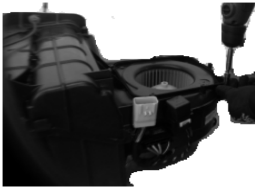
Remove the 14 screws holding the case halves together.
