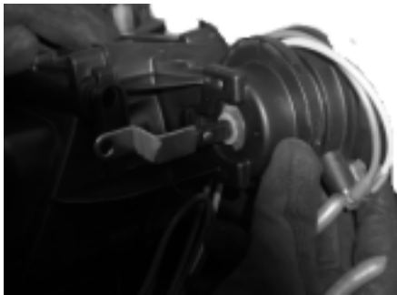
CAREFULLY remove actuator. Plastic parts break easily.
