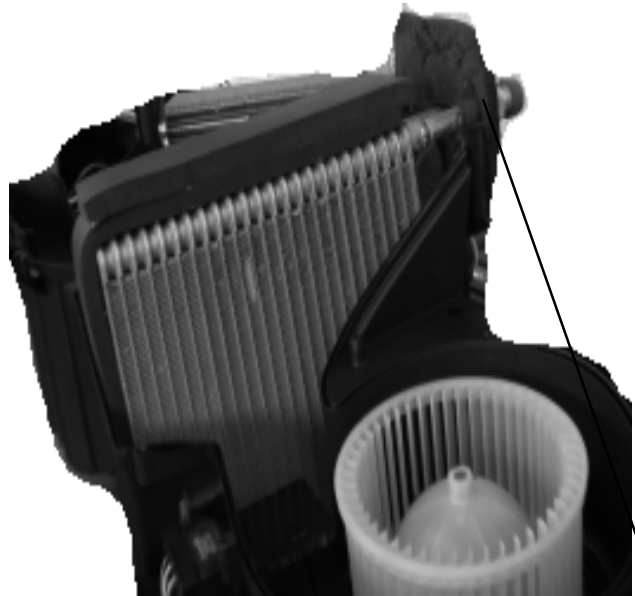
Carefully insert evaporator coil into the case. Cut a slot in the foam gasket for the tubes. Re-assemble in reverse order.
