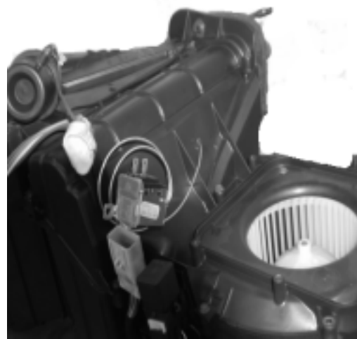
Drill a 1/8" hole and insert thermostat capillary tube into coil.
