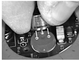
Figure 2. Installing the Sensor
