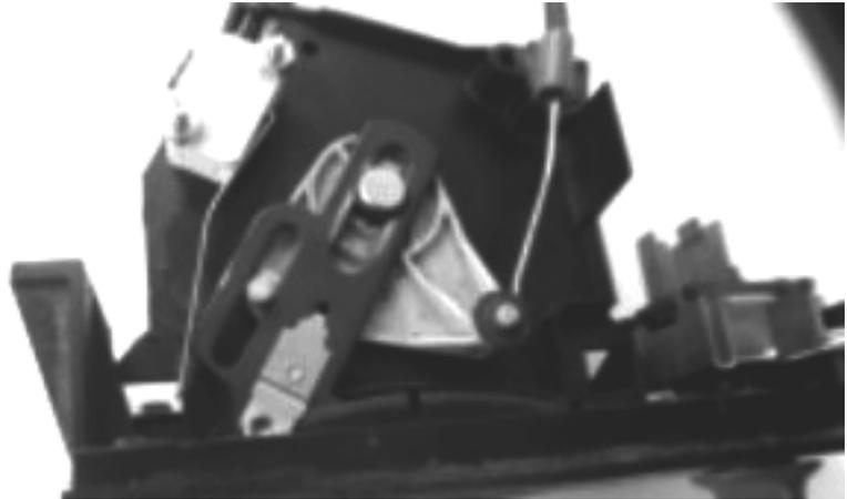
Using bolts and nuts provided, mount micro-switch in this position. Be sure arm swings free.
